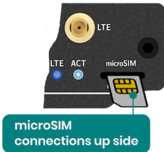
The card can be inserted the other way around and you can have the impression that you have inserted it correctly. So take a close look at the above drawing.
