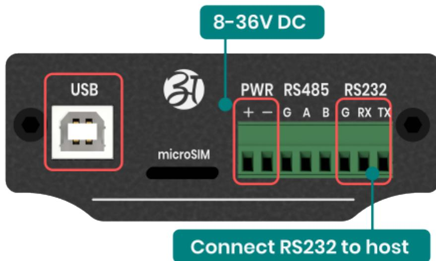
Remember that the modem's RX signal is combined with the host's TX signal, and the modem's TX signal is combined with the host's RX signal. That is, the signals are crossed. It is also necessary to connect common ground, or G.
