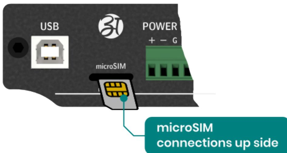
If by mistake you insert the card backwards then the card will be able to insert, but the modem will not work properly.
