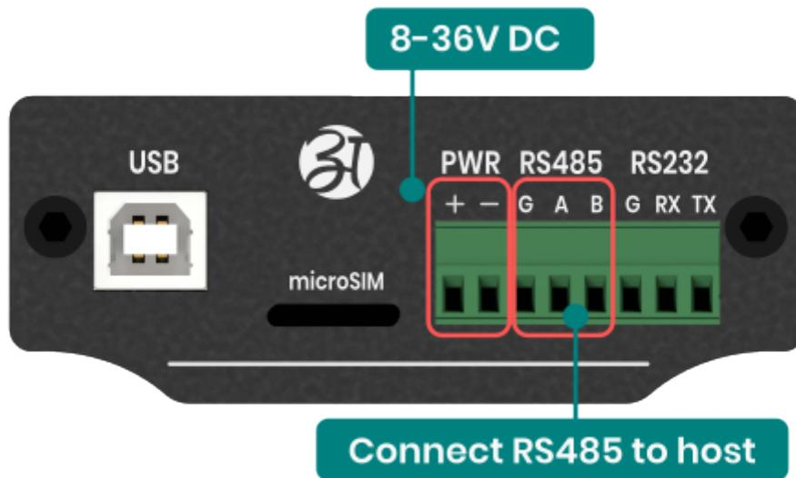
Always connect the modem's A signal to the host's A signal, and the modem's B signal to the host's B signal. Most of the time it is not necessary to connect the common ground, or G, signal, but it is good practice to connect it.
